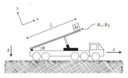
For this problem, use the x, y coordinate system shown in the figure. These coordinates are fixed with respect to the truck's bed, **not** to the ground.
