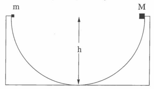
(1 point) (a) What is the total kinetic energy when the masses first touch (assume the size of the masses is much less than h)?
