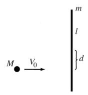
A ball of mass M hits a stick with moment of length l and mass m. The ball is initially traveling with velocity  $V_0$ , perpendicular to the stick. The ball strikes the stick at a distance d from its center. The collision is elastic. Find the resulting translational and rotational speeds of the stick, and also the resulting speed of the ball.
