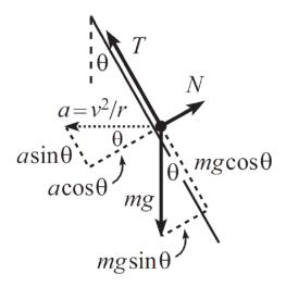
a. The free-body diagram is shown above. The net force produces the horizontal centripetal acceleration of  $a=v^2/r$ , where  $r=l\sin\theta$ . Let's work with axes parallel and perpendicular to the cone. Horizontal and vertical axes would work fine too, but things would be a little messier because the tension T and the normal force N would each appear in both of the F=ma equations, so we would have to solve a system of equations.
