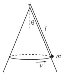
A mass m is attached by a massless string of length l to the tip of a frictionless cone. The half-angle at the vertex of the cone (angle between edge and central axis) is  $\theta$ . If the mass moves around in a horizontal circle at speed v on the cone, find:
