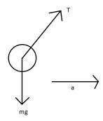
b. Since the car (and therefore the ball) is accelerating to the right with acceleration a, the net force cannot be zero. There must be a net force to the right. Since there is no vertical acceleration (the ball does not move up or down), the vertical forces must sum to zero.
