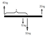
Using the figure above and Orsene as our reference point, we write down the torque balance:
