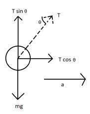
Balancing the forces in the vertical direction,  $T \sin \theta = mg \implies T = \frac{mg}{\sin \theta}$ .
