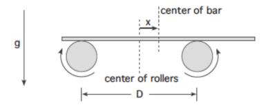
A bar of mass m and negligible height is lying horizontally across and perpendicular to a pair of counter rotating rollers as shown in the figure. The rollers are separated by a distance D. There is a coefficient of kinetic friction  $\mu$  between each roller and the bar. Assume that the bar remains horizontal and never comes off the rollers.
