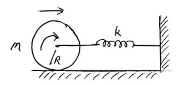
Attach a solid cylinder of mass M and radius R to a horizontal massless spring with spring constant k so that it can roll without slipping along a horizontal surface. Let us try to find the period of the simple harmonic motion for the center of mass of the cylinder.
