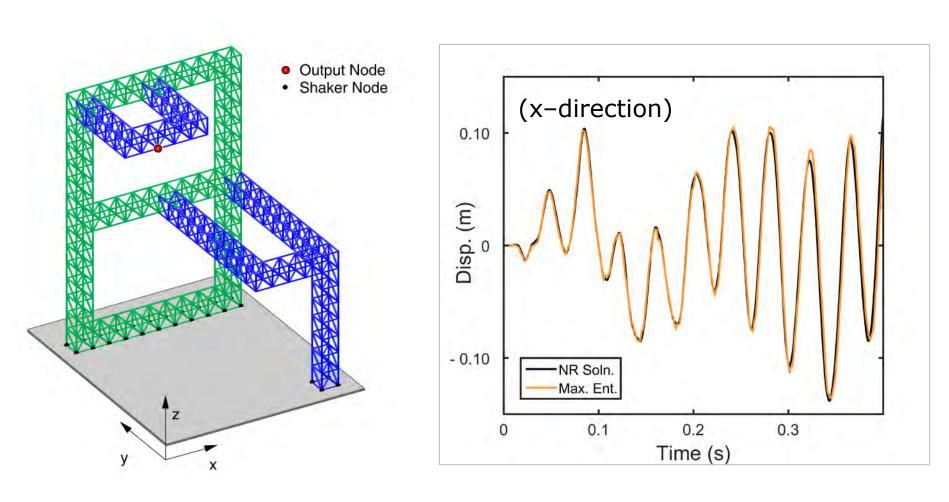
Data-Driven solution vs. direct Newmark solution
