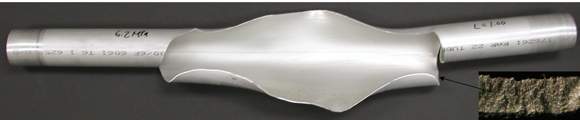
Detonation-driven Al-tube fracture (Shepherd et al., 2003)
