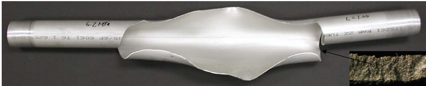
Detonation-driven Al-tube fracture (Shepherd et al., 2003)
