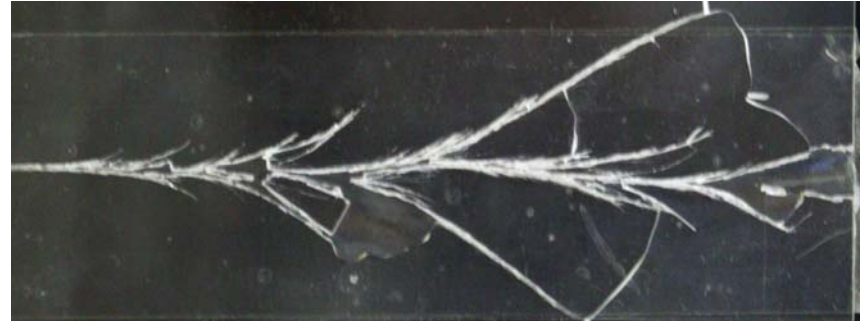
Dynamic crack branching (Fineberg and Sharon, 1992)
