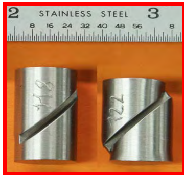
Shear Compression Specimen (SCS)
