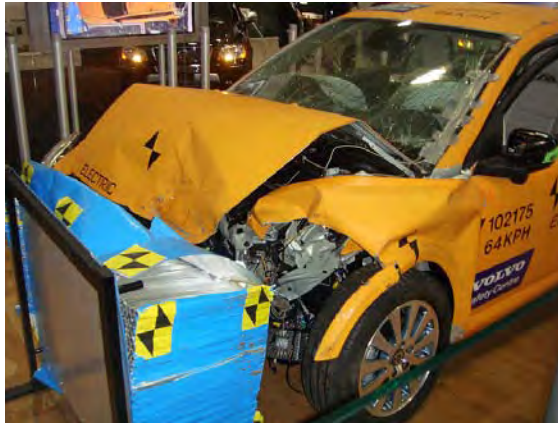
Frontal crash test of Volvo C30
