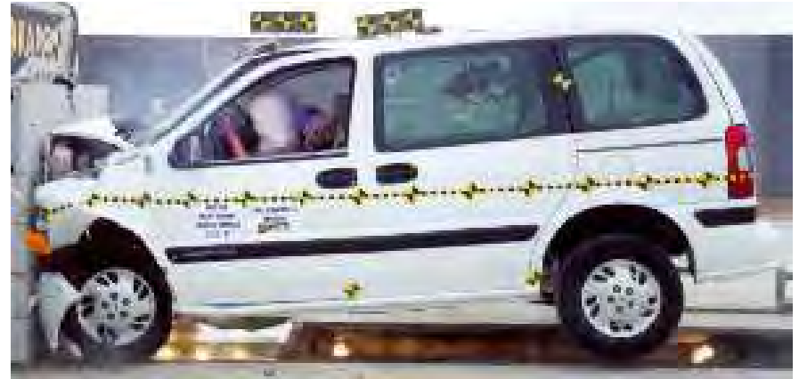
Frontal crash test of Chevrolet Venture
