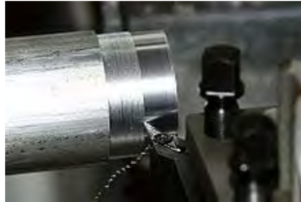
Lathe cutting metal from workpiece
