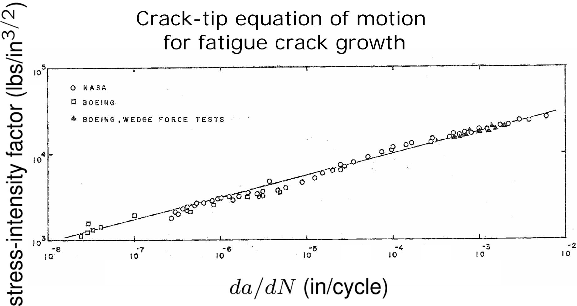
Crack-growth data for 2024-T3 aluminum alloy
