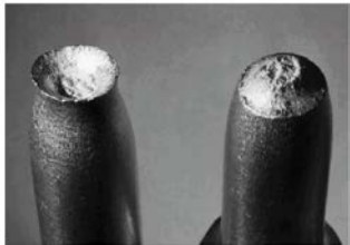
Cup-cone ductile fracture
