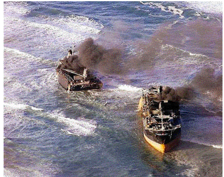
Failure of the New Carissa, on February 3, 1999, as a result of stress-corrosion cracking caused by extreme heat from burning, cyclic bending and seawater.
