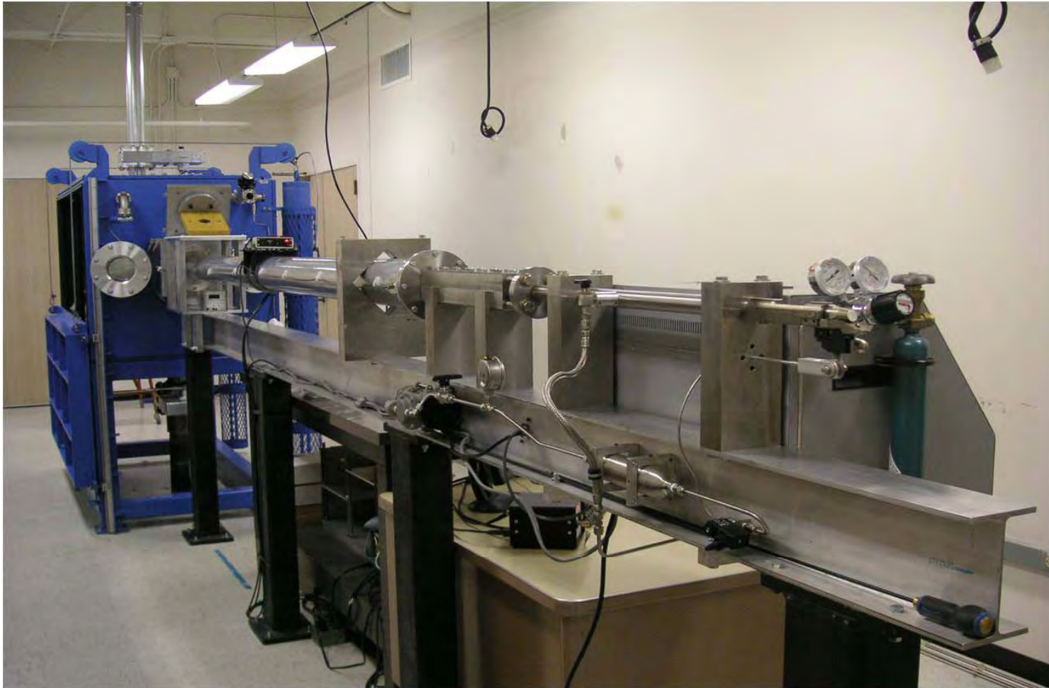
Caltech's Small Particle Hypervelocity Impact Range facility (Prof. A.J. Rosakis, Director)
