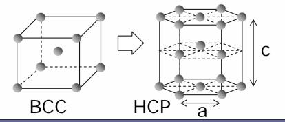
A strong shock wave will induce phase transitions producing complicated microstructure.
