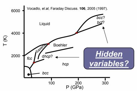
Ground state ferromagnetic *bcc* undergoes a *martensitic* phase transformation to non-magnetic *hcp* at ~10 GPa.
