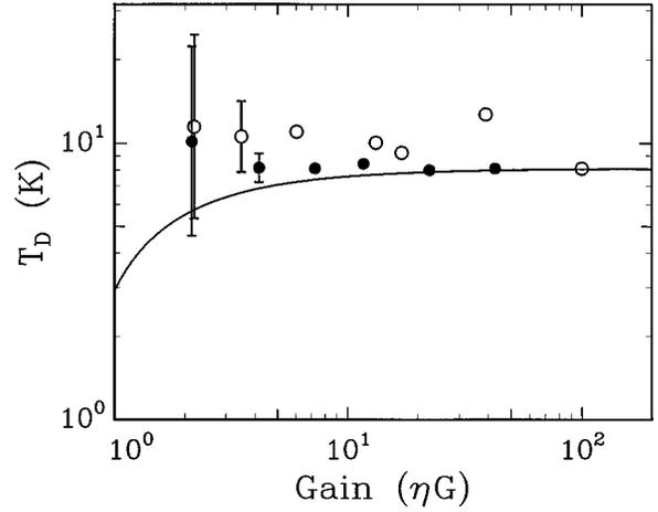
FIG. 1. The difference between the pump-on noise and the reference noise referred to input using the single sideband power gain  $\eta G$ . The error bars indicate uncertainty in the data due to detector saturation effects. Open circles represent data taken below threshold; filled circles represent data taken above threshold. The solid curve represents the theoretical prediction.
