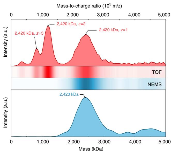
**Figure 2 | NEMS-MS greatly clarifies the spectrum.** Spectra for a nanocluster population with a mean mass of around 2,420 kDa acquired by both TOF and NEMS-MS. The TOF data was smoothed by applying a Savitsky–Golay filter. While multiply charged particles generate several peaks in the TOF-MS spectrum, the NEMS directly weighs the particle masses, yielding a single peak.
