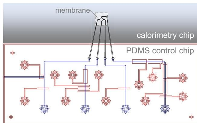
**Fig. 2.** Microfluidic layout. Pneumatically controlled PDMS microfluidics chip mated to parylene microfluidics on the calorimeter chip. The PDMS control layer (red) contains valves and peristaltic pumps. The PDMS flow layer (blue) is connected to the parylene channel (black) through an SU-8 via. Four injection pumps (containing large area valves) are built in the right upper corner.
