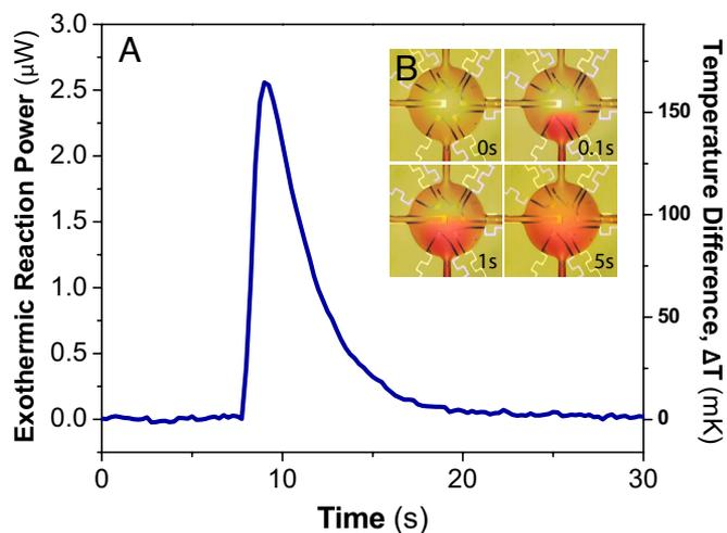
**Fig. 5.** Enthalpy of mixing measurement. (A) Heat of methanol dilution. A total of 1.4 nL of 14.7% methanol–water solution was mixed with 2.1 nL of water. (B) Visualization of the diffusive mixing process, enabled by the injection of red dye into the chamber filled with water.
