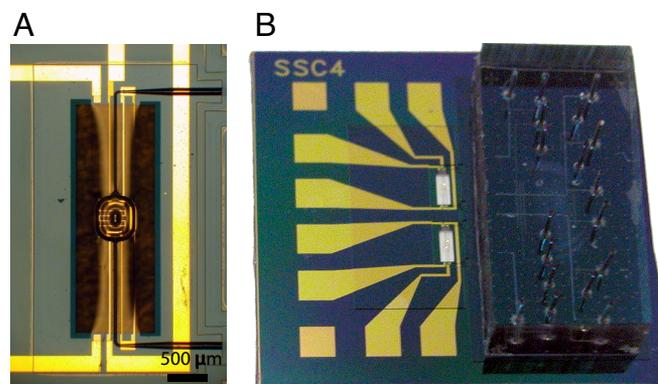
**Fig. 6.** Microscale flow calorimeter. (A) Parylene microfluidics and electronic sensor fabricated onto a parylene bridge structure. The measurement chamber is located at the middle of the bridge. (B) Flow calorimeter chip ( $3 \times 3 \text{ cm}$ ) with two identical measurement chambers (located at the transparent area at the center) for differential measurement.
