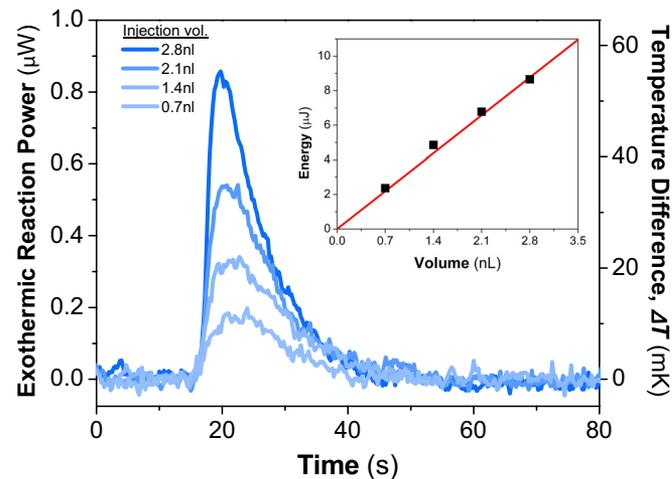
**Fig. 4.** Calorimetric signature of urea hydrolysis by urease. Calorimetric response after the injection of various volumetric aliquots of 50 mM urea solution into the chamber prefilled with urease solution. Four separate measurements are plotted on the same graph for comparison. (Inset) The total energy of reaction. The red line shows the expected energy of reactions deduced from the heat of reaction,  $\Delta H = 61$  kJ/mol.
