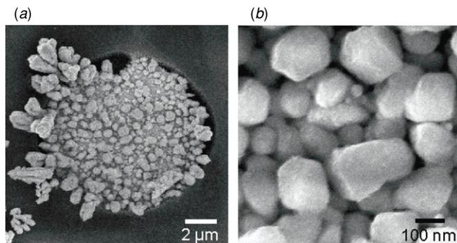
**Figure 7.** (a) Electron micrograph of a gold-electrodeposited microelectrode after a 9 day PBS immersion test. This site had an impedance of  $0.65 \text{ M}\Omega$  on the final day. (b) Close-up of the surface of an electrodeposited electrode.
