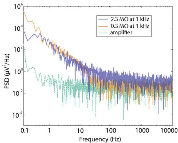
**Figure 9.** Noise power spectral density (PSD) of two gold microelectrodes ( $100 \mu\text{m}^2$  geometric area) with different impedance values. The lowermost trace represents the noise PSD from the shorted amplifier.
