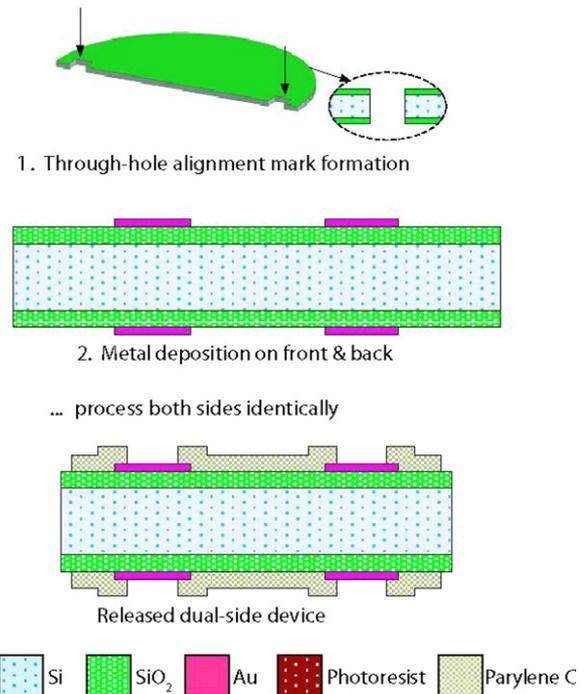
**Figure 3.** Modified process flow for fabricating dual-side devices on ultra-thin silicon substrates. The etching of through-holes is essential for achieving precise front-to-back feature alignment. Once metal has been evaporated on both sides, the parylene and oxide etch processes are carried out twice before the final DRIE step. The recording sites contain separately addressable leads on each side.
