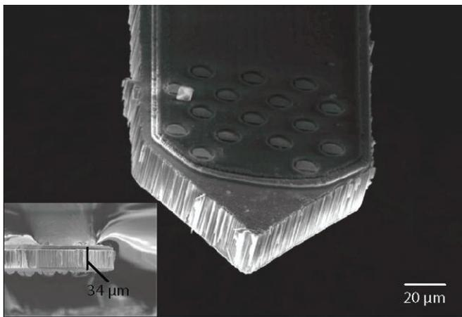
**Figure 5.** SEM micrograph of the tip of a dual-side neural probe. The total thickness of this structure, indicated by the cross-sectional view in the inset, is  $34 \pm 1 \mu\text{m}$ , which includes the ultra-thin substrate ( $\sim 28 \mu\text{m}$  before oxidation, manufacturer's specification =  $25 \pm 5 \mu\text{m}$ ) and a stack of  $2 \mu\text{m}$  thick thermal oxide and  $3 \pm 1 \mu\text{m}$  thick parylene-C film on each side.
