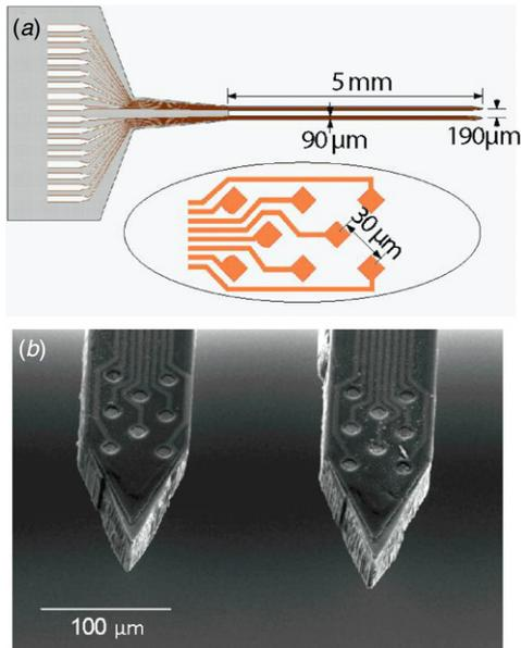
**Figure 2.** (a) Structure of a typical neural probe. This device contains two 5 mm long shafts. The inset shows the recording electrode arrangement. (b) SEM image of the tip of a fabricated probe. The gold electrodes have an area of  $100 \mu\text{m}^2$ , and the shafts have a thickness of  $50 \mu\text{m}$ .
