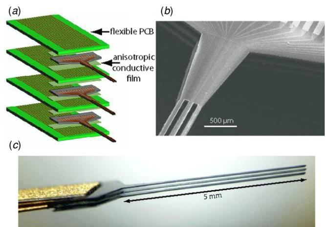
**Figure 6.** (a) Flip-chip assembly scheme for connecting the silicon devices with PCBs. (b) SEM micrograph of the rear section of a  $50 \mu\text{m}$  thick shaft array showing the multilayer stacked structure. Adjacent layers have a spacing of  $100 \mu\text{m}$ , which is set by the thickness of the flexible cable. (c) Side view of the  $50 \mu\text{m}$  thick shaft array showing that the shafts are stress balanced and are able to retain approximately constant relative spacing.
