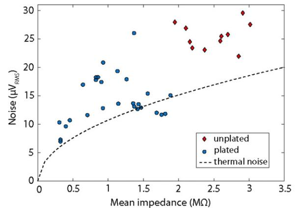
**Figure 10.** Root-mean-square noise at the electrode–fluid interface as a function of the mean impedance. The measurement bandwidth is 100–7000 Hz, and uncertainty in  $Z$  and  $\delta V$  is  $\sim 10\%$  (error bars not shown). Blue circles and red diamonds represent electrodeposited and unplated gold electrodes, respectively. The thermal noise for a resistor with  $R = Z$  is also calculated (dashed line).
