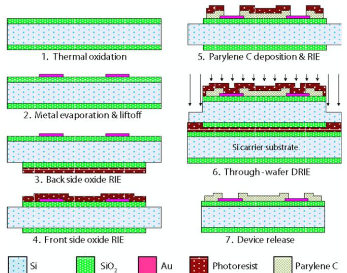
**Figure 1.** Fabrication process flow for single-side neural probe array built from ultra-thin silicon substrates. Each step relies on the use of a rigid supporting wafer to maintain structural integrity of the device substrate.
