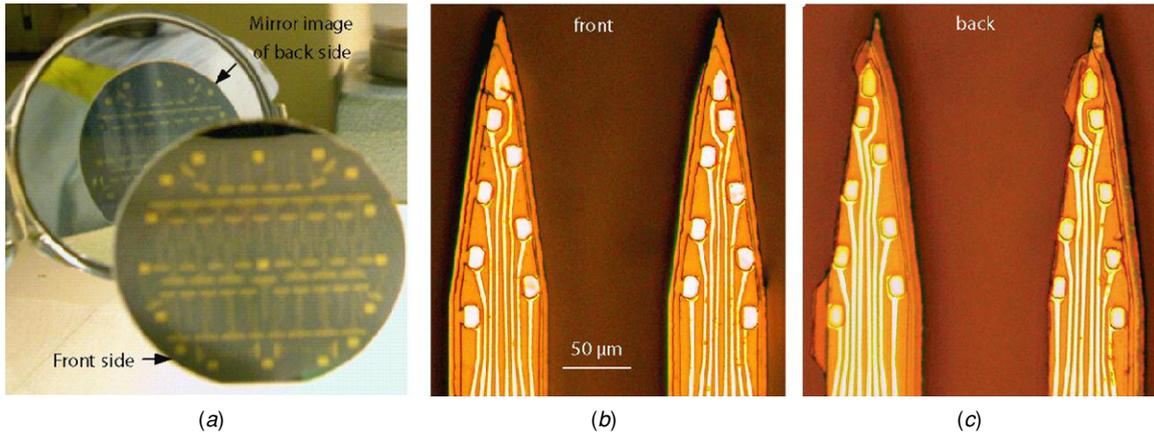
**Figure 4.** (a) The dual-side fabrication process is implemented on a 50 mm wafer. The transparent quartz carrier wafer is not visible. (b) Front and (c) back views of a representative finished device showing identical patterns. The overhanging structures on the left side of the shafts in (c) consist of SiO<sub>2</sub> that is displaced by up to 10 μm from the Si shaft due to slight misalignment of features between the front and backsides.
