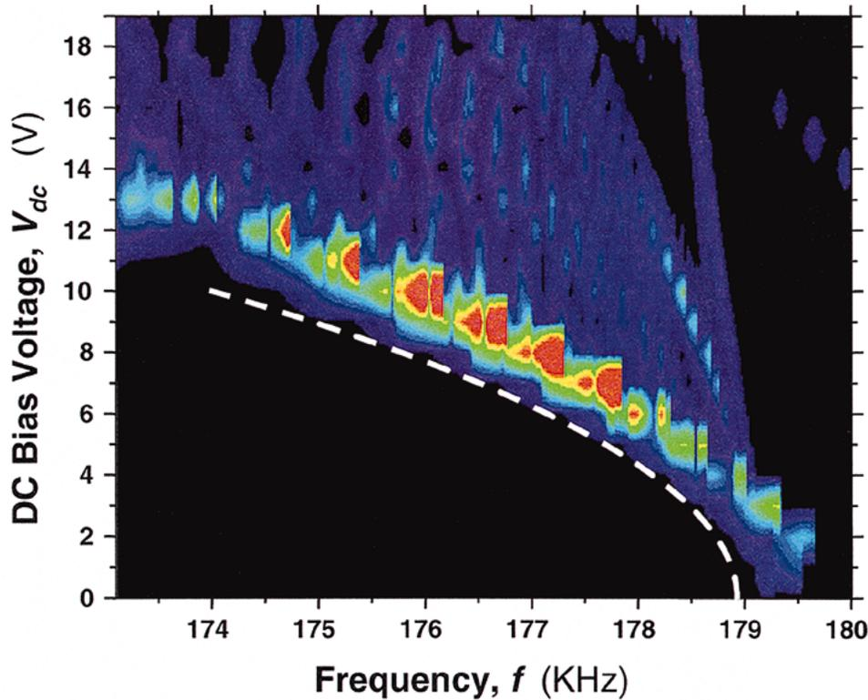
Fig. 5. A color map showing relative signal intensities measured at the lock-in amplifier operating in a  $2f$  mode. The dependence upon both the voltage  $V_{dc}$  and the frequency of the ac voltage  $f$  are shown. The wavelength is tuned to the diffraction peak, namely  $\lambda = 1582$  nm. The dashed white line shows a fit to the measured lower bound frequency  $f_b$  of the band.
