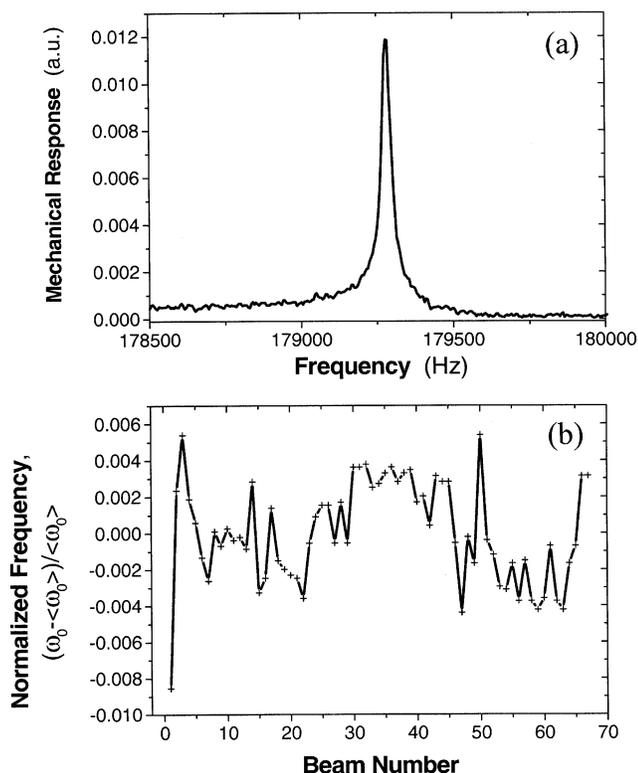
Fig. 2. (a) Response peak of an individual beam with a resonance frequency of 179.28 KHz. (b) Normalized resonance frequencies of all beams in the array  $(\omega_0 - \langle \omega_0 \rangle) / \langle \omega_0 \rangle$  where  $\langle \omega_0 \rangle$  is the average value.
