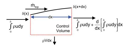
We define a control volume between x and x + dx, bounded by the surface of the plate and extending to the edge of the boundary layer. Continuity (conservation of mass) tells us that
