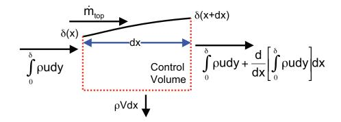
We define a control volume between x and x + dx, bounded by the surface of the plate and extending to the edge of the boundary layer. Continuity (conservation of mass) tells us that
