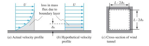
(a) The idea here is that at each location, the boundary layer displacement thickness effectively reduces the area of uniform flow. Location 2 has a smaller effective flow area than location 1 (because  $\delta_{D2} > \delta_{D1}$ ). From mass conservation, this tells us that the uniform velocity at 2 will be higher.
