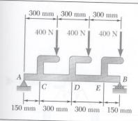
Draw the shear and bending-moment diagrams for the beam AB, and determine the maximum absolute values of the shear and bending moment.
