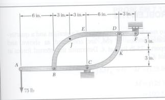
Two members, each consisting of a straight and a quarter-circular portion of rod, are connected as shown and support a 75-lb load at A. Determine the internal forces at Point J.
