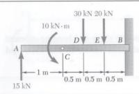
For the beam and loading shown, (a) draw the shear and bending-moment diagrams, (b) determine the maximum absolute values of the shear and bending moment.
