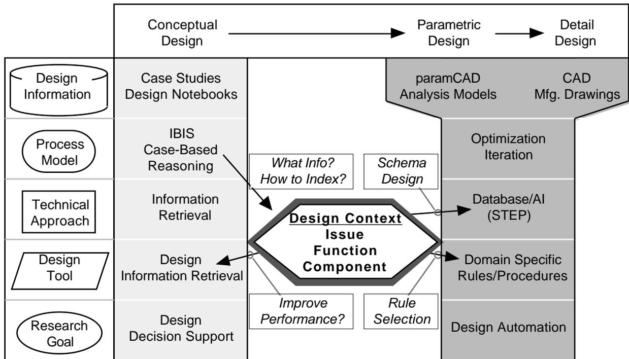
**Figure 1** Informal and formal strategies for supporting (respectively) early and late stages of design both depend on formalization of design context. Conceptual design is targeted for information retrieval techniques. Parametric and detail stages might take advantage of formalization through database or knowledge-based methods. Design context is a primary measure of design situation similarity whether it is used for information retrieval, database querying, or knowledge-based rule selection.
