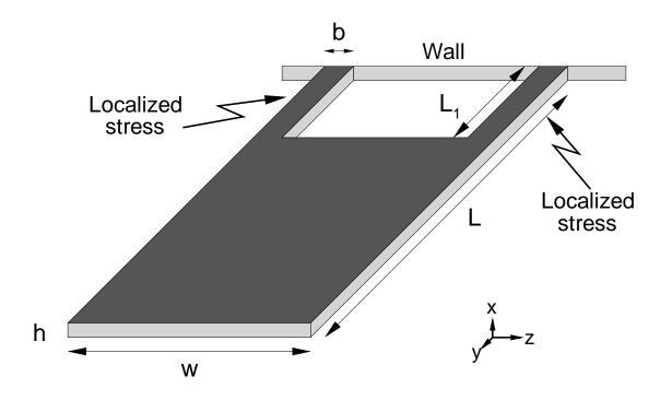
**Dimensions:**  $L = 3\mu$ , W = 100nm,  $L_1 = 0.6\mu$ , b = 33nm **Material:**  $\rho = 2230$ Kg/m<sup>3</sup>,  $E = 1.25 \times 10^{11}$ N/m<sup>2</sup>
