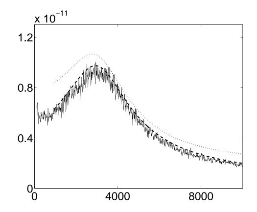
$232.4\mu \times 20.11\mu \times 0.573\mu$  Asylum Research AFM (Clarke et al., 2005) Dashed line: calculations from fluctuation-dissipation approach Dotted line: calculations from Sader (1998) approach
