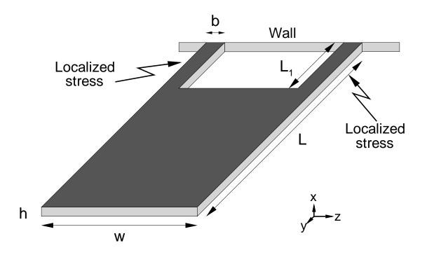
**Dimensions:**  $L = 3\mu$ , w = 100nm, t = 30nm,  $L_1 = 0.6\mu$ , b = 33nm **Material:**  $\rho = 2230$ Kg/m<sup>3</sup>,  $E = 1.25 \times 10^{11}$ N/m<sup>2</sup>
