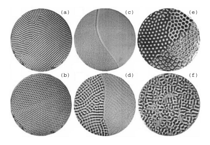
Vertically shaken layer of tiny balls (layer depth 1.2mm, ball diameter 0.15-0.18mm) [From Melo, Umbanhowar, and Swinney]
