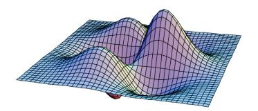
Gaussian Derivative filter  $D_x D_y^2 G_\sigma(x,y)$  with  $\sigma_x = \sigma_y = 2$
