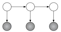
Fig. 4.2 The HMM of length three.
