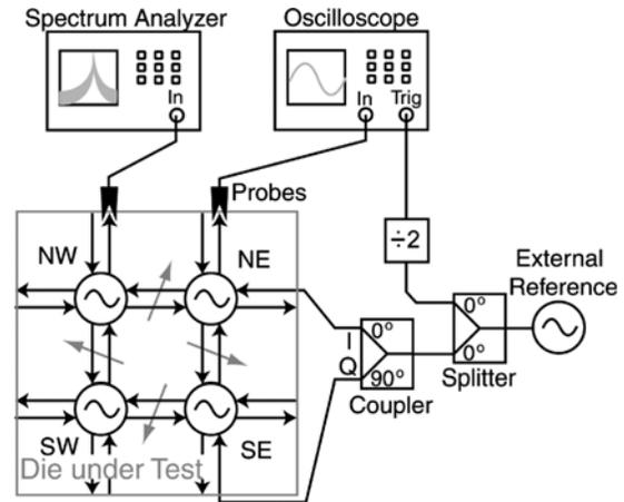
Fig. 13. Testing scheme for the coupled-oscillator array.
