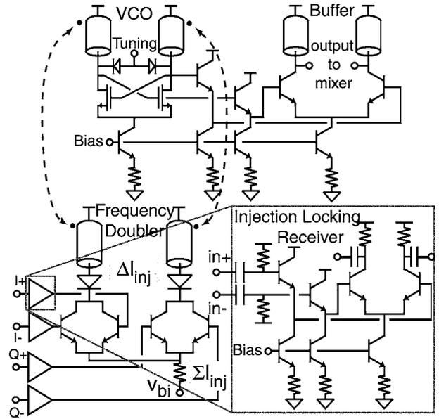
Fig. 6. Injection locking and VCO topology.
