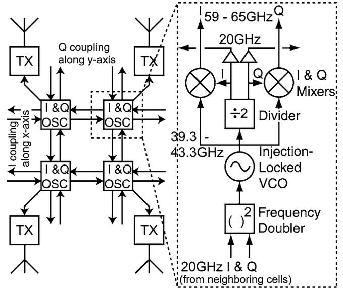
Fig. 3. Coupled-oscillator schematic. The oscillators are coupled along two dimensions. The coupling network operates at one-third the carrier frequency.
