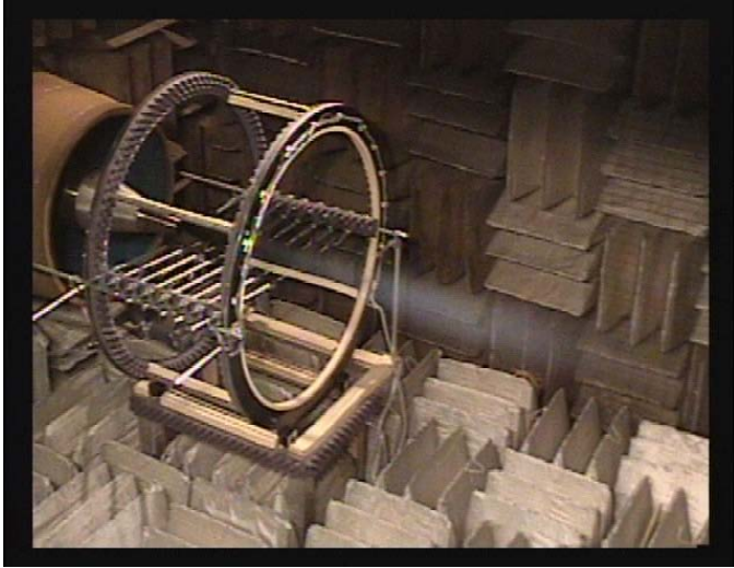
Figure 3. Rotating array installed in UTRC ART: a) supersonic jet noise study, b) view looking upstream into open jet with rotating array in vertical position
