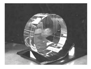
Fig. 5.18. A LIGO mirror, which will be seen to behave quantum mechanically in LIGO's upgraded interferometers, in 2008
