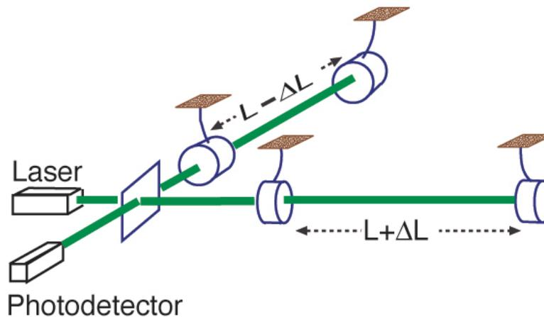
Figure 9. A laser interferometer gravitational-wave detector.
