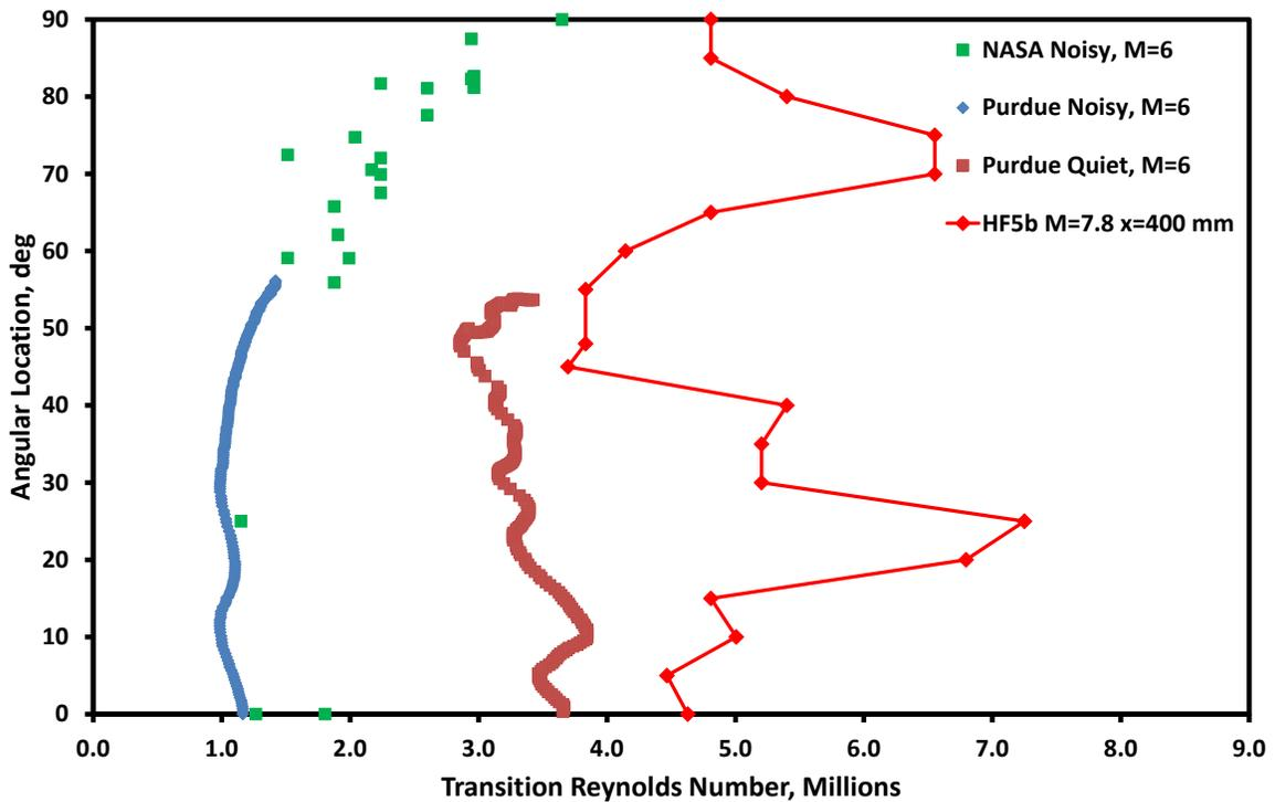
Figure 7 Noisy and quiet wind tunnel transition compared to flight transition.
