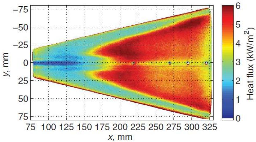
Figure 9 Heat transfer contours derived from temperature-sensitive paint image from Purdue wind tunnel  $M=6$ ,  $Re=10.2 \times 10^6 / m$ ,  $\alpha=0^\circ$ , noisy flow (Ref. 39).
