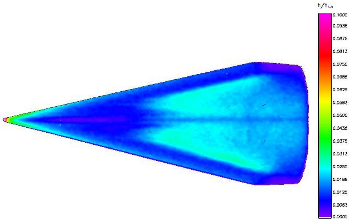
Figure 8 Heat transfer contours derived from thermographic phosphor image from LaRC Run 8.  $M=6$ ,  $Re=9.5 \times 10^6 / m$ ,  $\alpha=0^\circ$ . Enlarged image extracted from Ref. 36.
