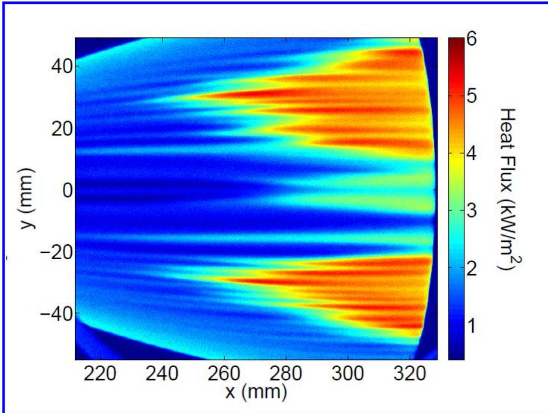
Figure 6 Heat transfer for HIFiRE-5 derived from infrared imaging,  $M=6$ ,  $Re=12.3 \times 10^6/m$ , quiet flow, Purdue wind tunnel (Ref. 34).
