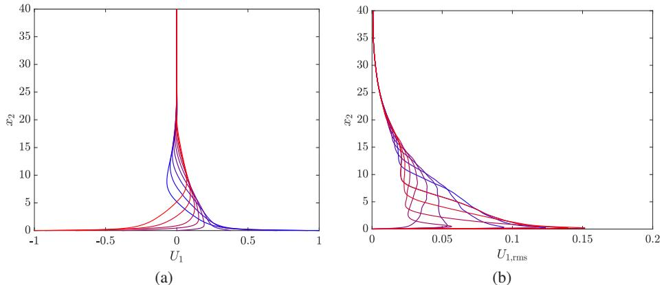
Figure 7: (a) Mean streamwise velocity profile and (b) streamwise r.m.s. velocity from  $t\Omega = 0$  (blue) to  $t\Omega = \pi$  (red). The profiles shown are at  $t\Omega = n\pi/8$ ,  $n = 0, 1, \dots, 8$ .
