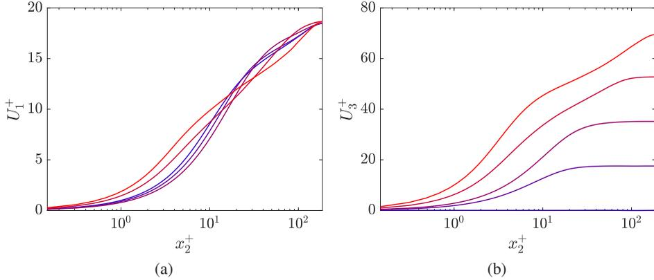
Figure 11: Mean (a) streamwise and (b) spanwise velocity profile from  $t = 0$  (blue) to  $t = 2.34$  (red). The times shown are  $t = 0, 0.58, 1.17, 1.76, 2.34$ . Data taken from Lozano-Durán *et al.* (2021). Time  $t$  is nondimensionalised with  $u_{\tau,0}/\delta$
