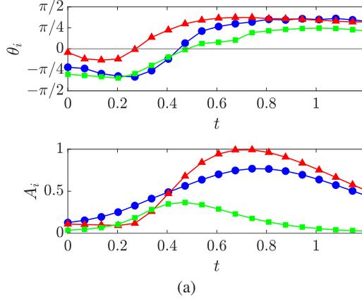
Figure 6: Mode angle (top) and magnitude (bottom) of the principal response mode as a function of time. The streamwise component of the mode is represented by  $\bullet$  (blue), the wall-normal component by  $\blacksquare$  (green) and the spanwise component by  $\blacktriangle$  (red).
