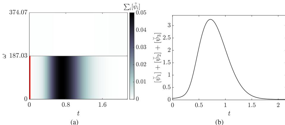
Figure 4: (a) Inverse wavelet-transformed principal response mode for channel flow at  $Re_\tau = 2000$  and  $k_1 = k_3 \approx 8.98$  under windowed forcing, in the frequency-time plane. The forcing window is highlighted in red. (b)  $x_2$ -integrated total energy of the inverse wavelet-transformed principal response mode.
