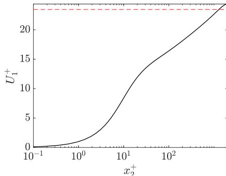
Figure 3: Mean streamwise velocity profile for channel flow at  $Re_\tau = 2000$ . The dashed line corresponds to the upper bound of the frequency band covered by the chosen wavelet, mapped to streamwise velocities using  $U_1 = \omega/k_1$ .
