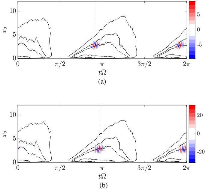
Figure 9: Real part of (a)  $\check{\phi}_1$ , and (b)  $\check{\psi}_1$  for the turbulent Stokes boundary layer. The black contour lines are  $U_{1,rms}$  with the levels indicating 30%, 50%, 75%, 95% of its maximum value. The vertical dashed lines show the times of the amplitude peak for the input mode ( $t\Omega = 2.84$ ) and output mode ( $t\Omega = 3.03$ ).
