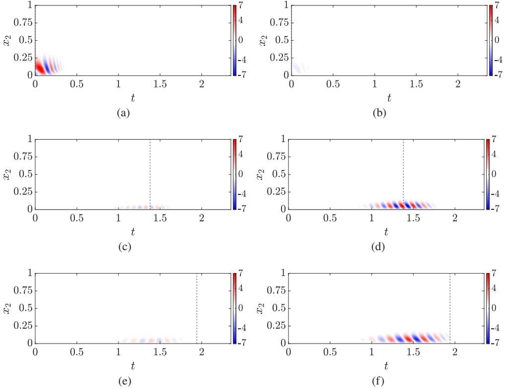
Figure 13: Real part of  $\check{\psi}_1$  (left) and  $\check{\psi}_3$  (right) for the turbulent channel subject to a spanwise pressure gradient. The chosen spatial scales are (a, b)  $\lambda_1^+ = 1000$ ,  $\lambda_3^+ = 100$ , (c, d)  $\lambda_1^+ = 189$ ,  $\lambda_3^+ = 1890$ , and (e, f)  $\lambda_1^+ = 297$ ,  $\lambda_3^+ = 2970$ . The vertical dashed lines mark (a, b)  $t = 0$ , (c, d)  $t = 1.38$ , and (e, f)  $t = 1.94$ .
