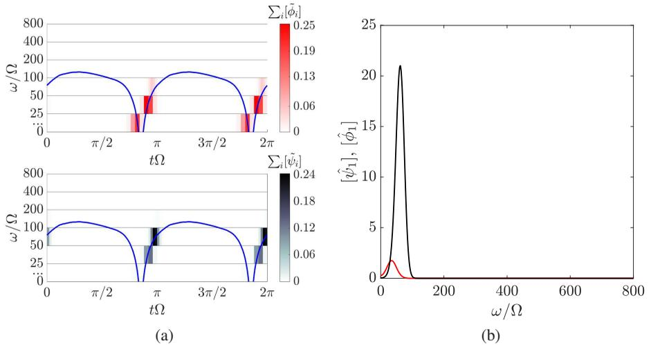
Figure 10: (a) Principal forcing (red, top panel) and response (black, bottom panel) modes in the time-frequency plane; the blue line indicates  $U_1 k_1 / \Omega$  at  $x_{2,avg}^{resp.} = x_{2,avg}^{forc.} \approx 0.071$ ; (b)  $x_2$ -integrated frequency content in the streamwise component of the forcing (red) and response (black) modes.
