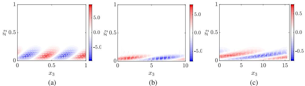
Figure 15: Principal response mode in the  $x_2 - x_3$  plane at (a)  $t = 0$ , (b)  $t = 1.38$ , and (c)  $t = 1.94$ , rotated by  $-\gamma$ . The contours represent the streamwise component; the arrows represent the velocity field in the wall-parallel plane and are colored according to  $\sqrt{|\psi_2|^2 + |\psi_3|^2} \text{sgn}(\psi_3)$ .
