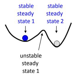
At Steady states, production rate = clearance rate
