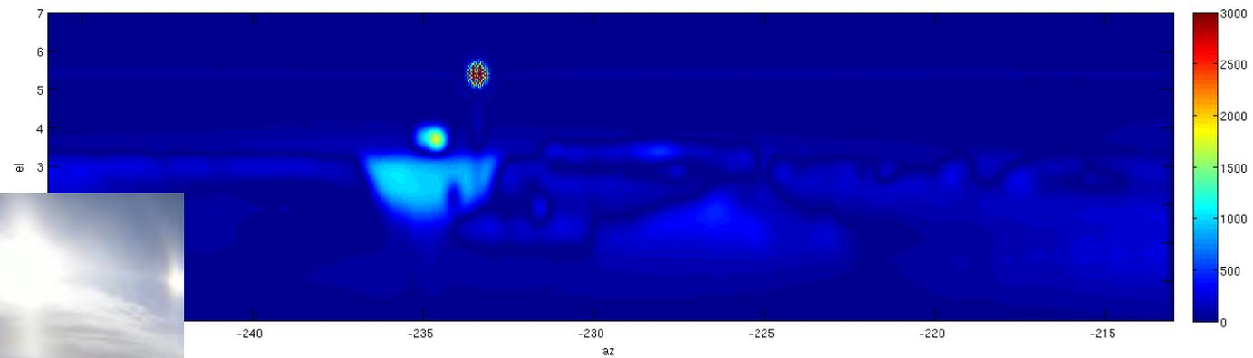
**ultra-deep beam calibrations:** BICEP3 viewing an amplified polarized calibration source over the ground shield using a mirror
