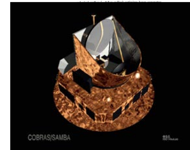
Figure 4 - Schematic COBRAS payload concept. The Gregorian optical system assumed in our performance simulation study is represented in white. The pointing effect from the spin axis (here assumed to be 1°) will be optimized during the summer study together with the details of the scan strategy. The ground antenna will have not as an appropriate angle to optimize absolute pickup and cooling efficiency. The last shows a schematic of the first phase array of feed horn feeds. Placing their apertures in a
