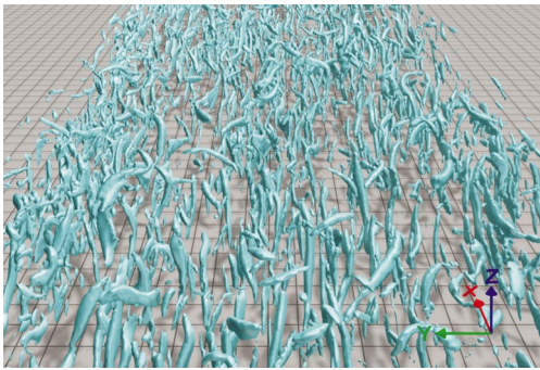
FIG. 1. Single-phase flow: vortical structures at t=60 .
