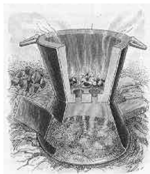
FIGURE 11. THE KENYAN CERAMIC JIKO (CUT-OUT VIEW)
