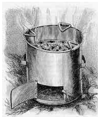
FIGURE 11. THE KENYAN CERAMIC JIKO (CUT-OUT VIEW)
