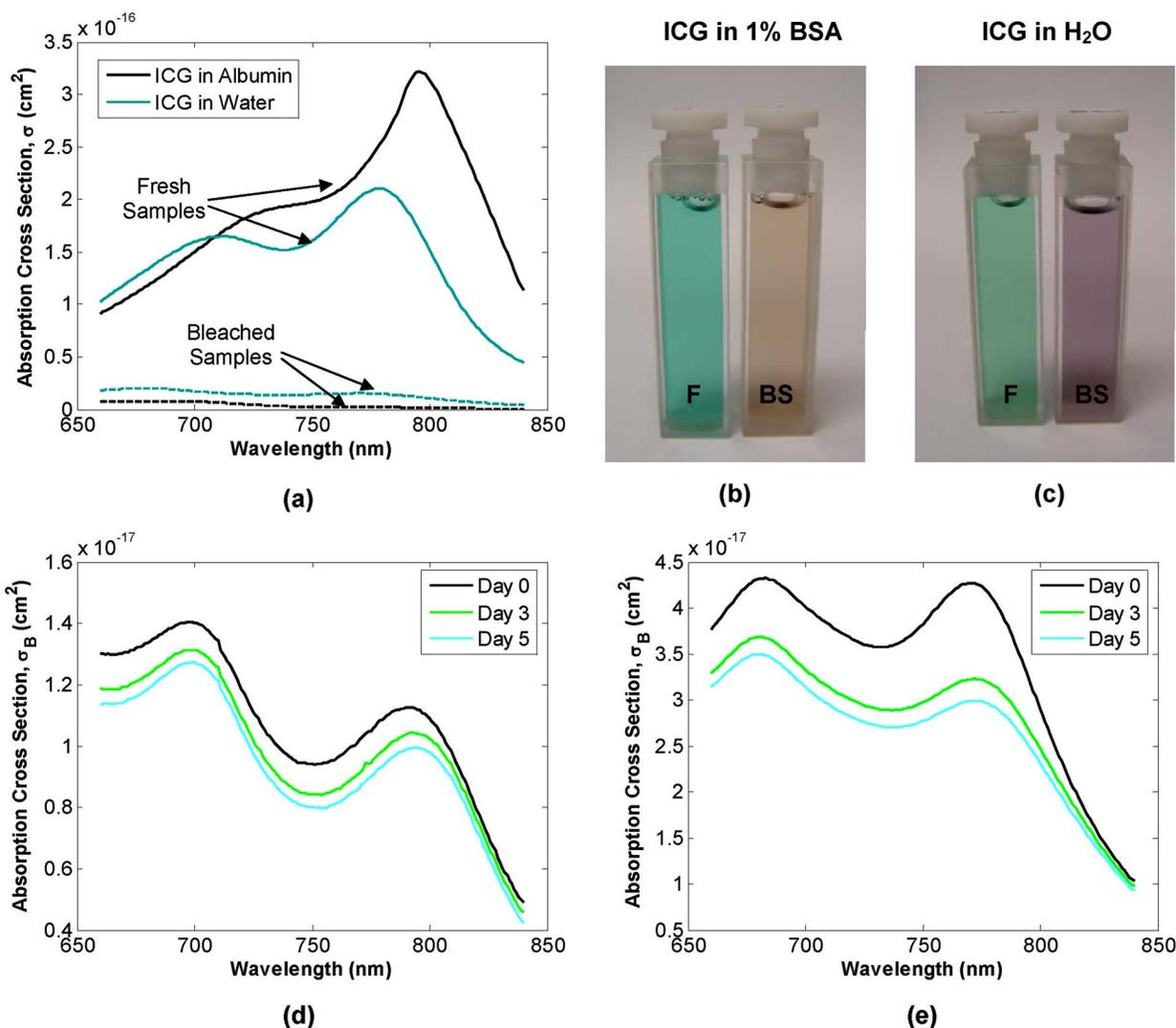
**Fig. 2** Shows (a) absorption cross-section spectra and (b) and (c) pictures of unbleached as well as bleached samples of ICG in 1% BSA and water. ICG concentration is  $50 \mu\text{M}$  in all the cases. (d) and (e) show absorption spectra of bleached samples of ICG in BSA and water, respectively, acquired at different times. F: fresh; BS: bleached sample.
