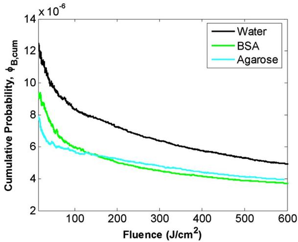
**Fig. 5** Cumulative probability  $\phi_{B,cum}$  for 50- $\mu$ M ICG in DI water, 1% BSA, and 0.8% agarose. The irradiance in all cases is 33.55 W/cm<sup>2</sup>.
