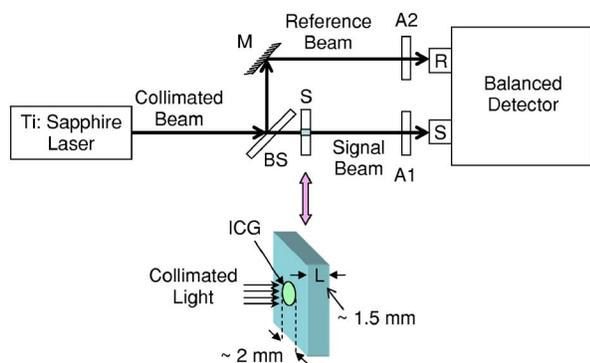
**Fig. 3** Experimental setup to study ICG photodegradation dynamics. BS: beamsplitter; M: mirror; Ai: *i*'th attenuator; R: reference beam; S: sample beam.
