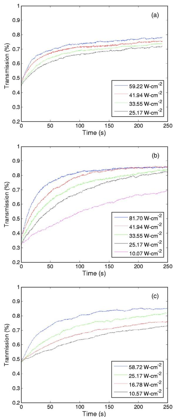
**Fig. 4** Transmission curves for 50  $\mu\text{M}$  ICG versus time in (a) DI water, (b) 1% BSA, and (c) 0.8% agarose for different illumination intensities (irradiance levels).
