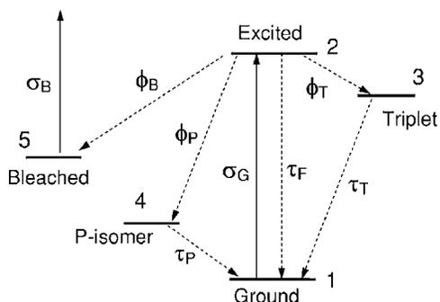
**Fig. 1** Schematic of electronic state diagram of ICG.  $\sigma_G$  is the ground state absorption cross section, whereas  $\phi_T$ ,  $\phi_P$ , and  $\phi_B$  are quantum yields of triplet ( $T$ ),  $P$ -isomer ( $P$ ), and bleached ( $B$ ) states.
