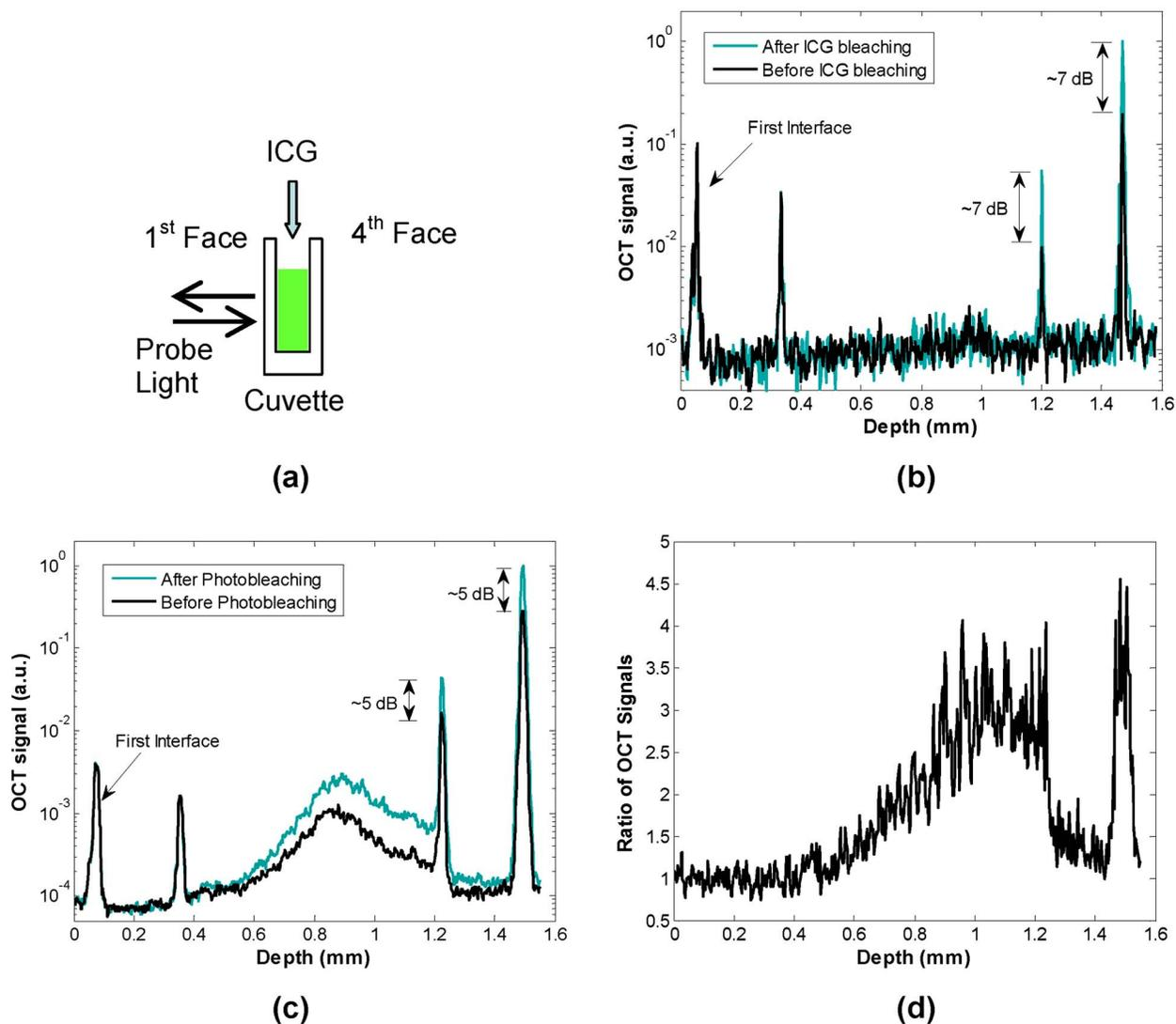
**Fig. 9** (a) Side view of a 0.84 mm path length cuvette used as a sample. (b) A-scans of the glass cuvette filled with 200  $\mu\text{M}$  ICG solution in 1% BSA before and after the photobleaching. (c) A-scans of the glass cuvette was filled with a mixture of 200  $\mu\text{M}$  ICG and 0.25% volume concentration 0.1  $\mu\text{m}$  latex microspheres before and after the photobleaching. (d) Ratio of the two A-scans is shown in (c).
