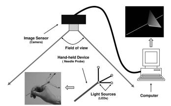
Fig. 1. Schematic of the tracking system. The left bottom inset is a photo of our prototype hand-held probe. The right top inset is a 3D rendering of the probe by the tracking system.
