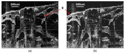
Fig. 4. (Color online) OCT images of a 54-stage *Xenopus laevis* tadpole specimen: (a) OCT image acquired by manually scanning without tracking correction and (b) OCT image acquired by manually scanning with tracking correction; g, gill pockets.
