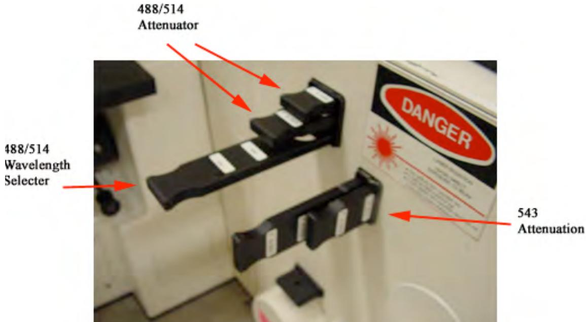
In “At” menu, set the left column to 1 and the right column to the number that matches the total laser line attenuation that results from the chosen attenuator positions (see tables below).
