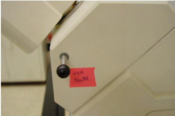
**A) Check Eye Shutter:** Directly below the eyepieces, on the right of the scope, there is a blackout slider for added protection during laser scanning. An internal, automatic shutter (that is activated when the LSM light path is selected) duplicates this slider.
