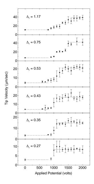
Figure 2. Tip velocities as a function of applied potential and supersaturation  $\Delta_1$ , for ice needles grown at T=-5 C. Horizontal dotted lines were drawn through the first and last data points to guide the eye.
