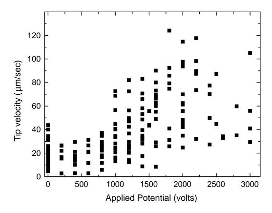
Figure 3. Tip velocities of growing iodine needle crystals as a function of the applied electrical potential. Each point represents the measurement of a single needle. Although the data show considerable scatter, there is clearly a large velocity increase above a threshold of  $\sim 1000$  volts, verifying the existence of this morphological instability for non-polar molecular systems.
