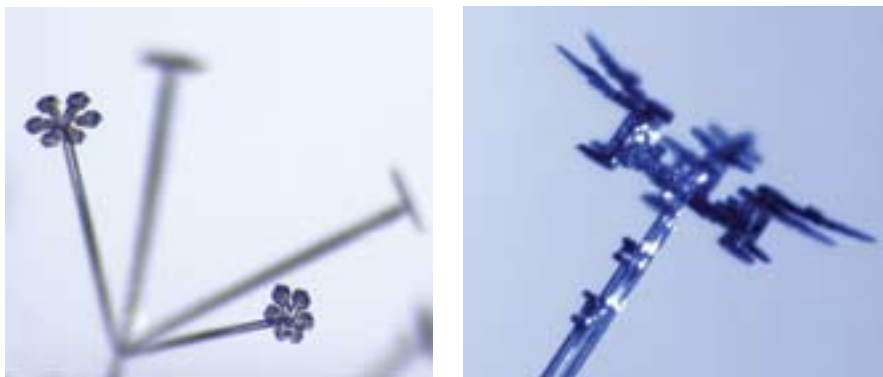
Figure 5. Laboratory-grown snow crystals offer the opportunity to explore in detail the combination of growth mechanisms and the different conditions under which they occur. Since experimental chambers cannot provide the same free-fall time as the atmosphere, it is desirable to grow supported crystals. One technique is to grow snow crystals on the tips of thin ice needles that sprout from an electrified wire (left). The strong electric field attracts water molecules in the air, greatly accelerating the needle's growth. When the electric charge is removed, crystal growth returns to normal. By controlling temperature and humidity, designer snowflakes can be created. For instance, a dendrite can be made to grow hollow columns at its points, then plates can be grown to cap each column, resulting in a shape that resembles a fancy chandelier (right). The series of temperature shifts required to produce such a form would be highly unlikely within a natural cloud bank.
