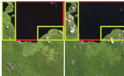
Figure 11: Satellite images taken from the New Britain rainforest in Papua Guina at 1989 (left) and 2000 (right). Red boxes identify the subframe used for the experiment, and green boxes identify the regions with higher associated weight in the weighted \ell_1 recovery. Image originally belongs to Royal Society for the Protection of Birds and was taken from the Guardian archive, an article on deforestation http://www.guardian.co.uk/environment/2008/jan/09/angeredredspecies.endangeredhabitats .
