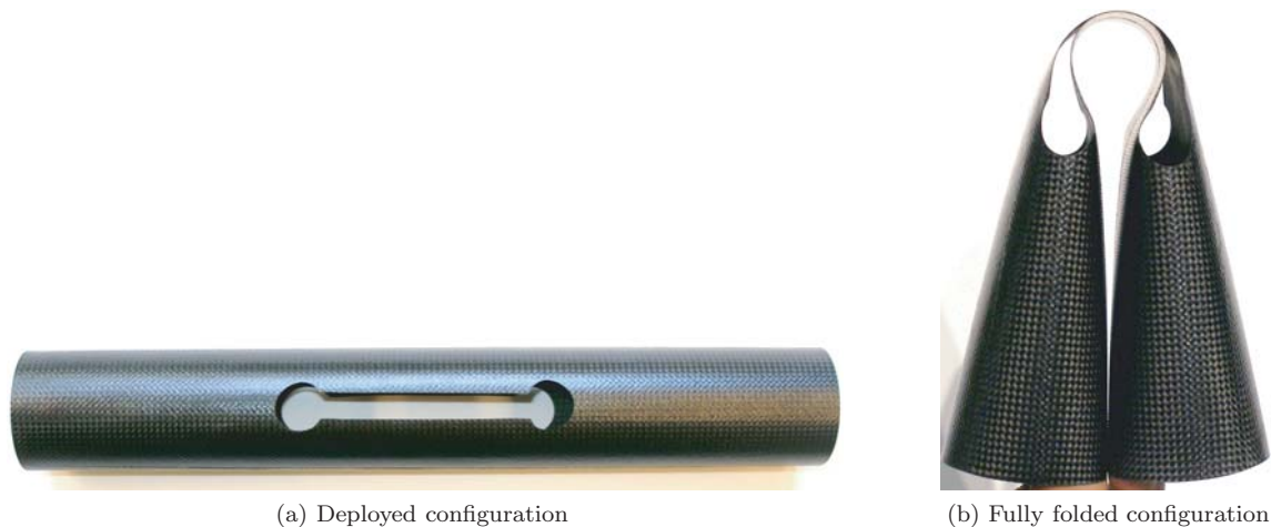
Figure 15: Tube hinge with SW=8 mm, D=15 mm and L=90 mm.
