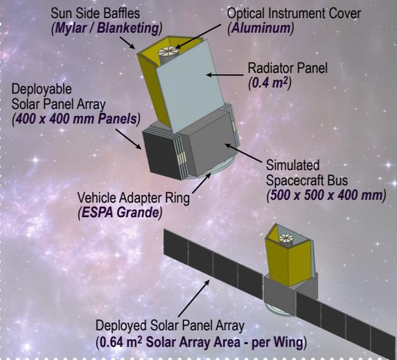
MISE provides a stable mid-IR telescope from space with a rideshare configured platform:
