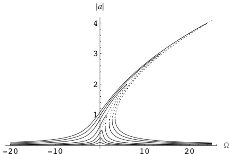
Amplitude v. frequency offset for different drives
