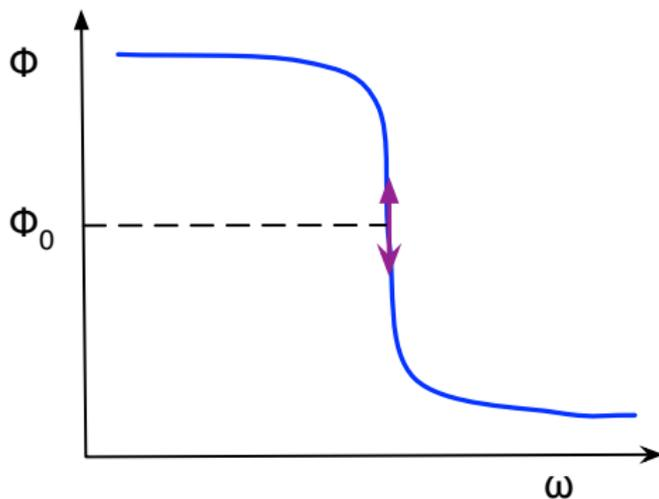
Frequency fluctuations of oscillator reduced by tuning to nonlinear critical point
