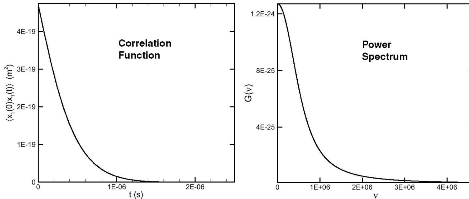
$1\mu\text{s}$  force sensitivity:  $K\sqrt{G_X(\nu) \times 1\text{MHz}} \sim 7\text{pN}$
