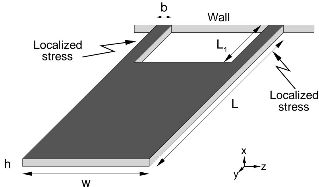
**Dimensions:**  $L = 3\mu$ ,  $w = 100\text{nm}$ ,  $t = 30\text{nm}$ ,  $L_1 = 0.6\mu$ ,  $b = 33\text{nm}$
