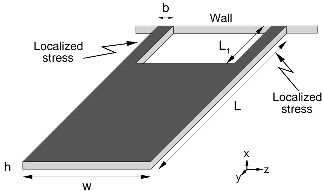
**Dimensions:**  $L = 3\mu$ ,  $W = 100\text{nm}$ ,  $L_1 = 0.6\mu$ ,  $b = 33\text{nm}$
